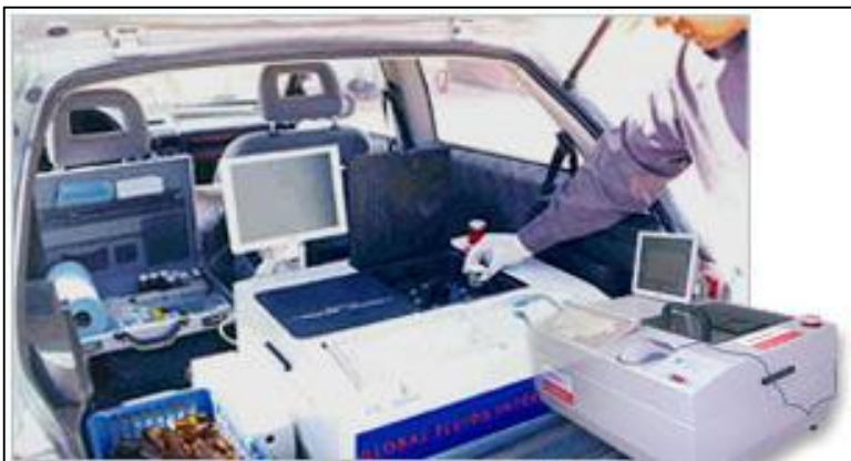
Figure 2: XRF used in field kept in backside of the Multi Utility Vehicle.
